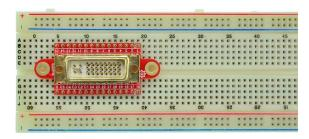
Figure 2: Example of connecting the DVI-IM-BO-V1AV on a breadboard
